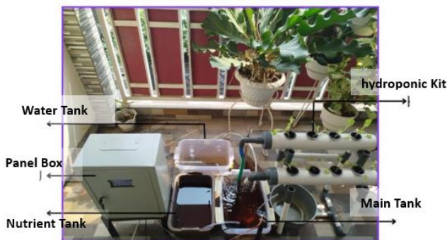
Figure 5. Realization of the Hydroponic System
