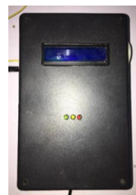
Picture 3. Panel Box Monitoring Control Water Level
