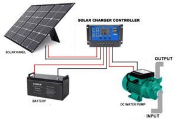
Figure 2. Solar water pump schematic
