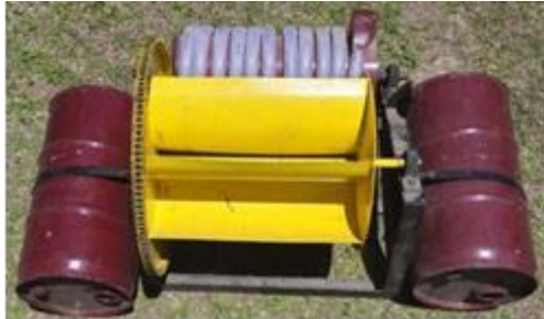
Figure 3. The water pump resembles Archimedes' spiral.
