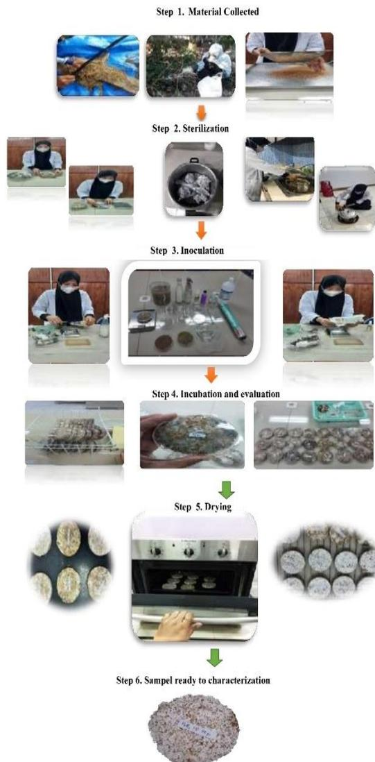
**Figure 1.** The procedure for making mycelium composite
